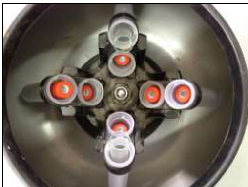
Figure 2: Centrifugation at 3000 rpm for 12 minutes.
